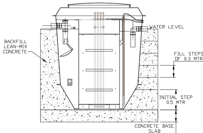
Step 7 Commence back filling with lean mix (for specifications Item 5, Introduction). The back fill must be evenly placed around the unit at all times and worked by hand up to a maximum level of 400mm above the base.
