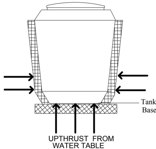
The local ground conditions must be taken into account when installing the unit. The amount of concrete backfill used must be sufficient to overcome the effects from up thrust of ground water.
