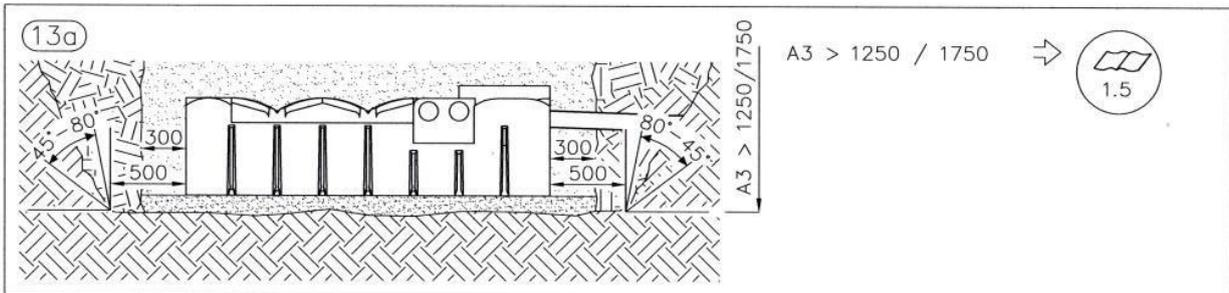
**4. Main dimensions and positions of the standard connections**
