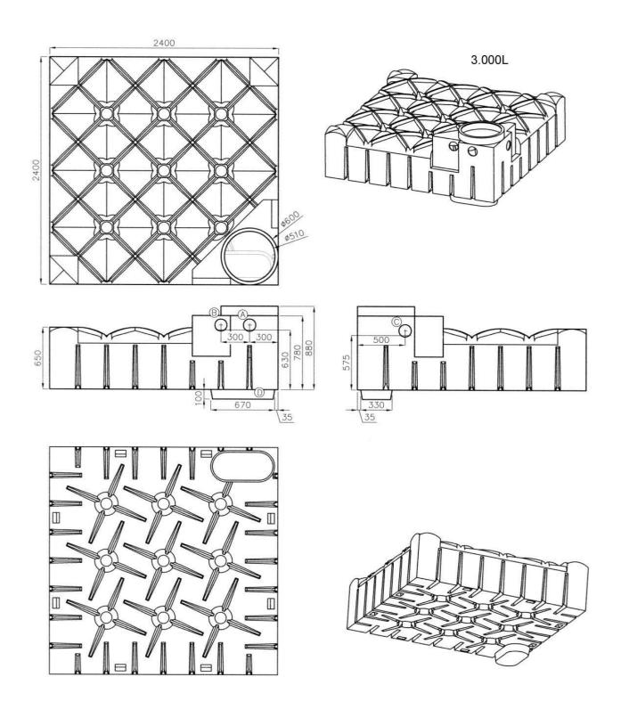
Rainwater utilisation: A/B Connection inflow/connection service pipe DN 100; connection overflow DN 100; D pump basin, see front page \* height tank shoulder
