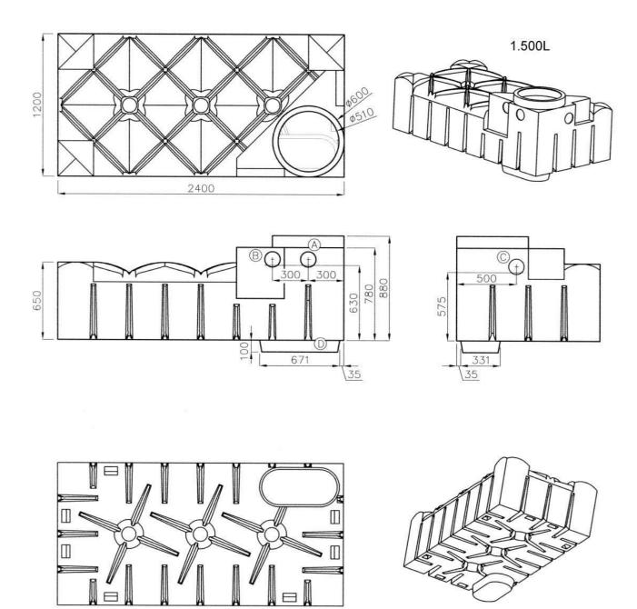
Rainwater utilisation: A/B Connection inflow/connection service pipe DN 100; connection overflow DN 100; D pump basin, see front page \* height tank shoulder
