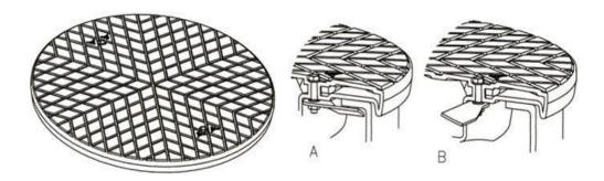
A safety latch closed B safety latch opened
