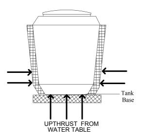
The local ground conditions must be taken into account when installing the unit. The amount of concrete backfill used must be sufficient to overcome the effects from up thrust of ground water.
