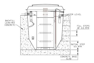
Step 7 Commence back filling with lean mix (for specifications Item 5, Introduction). The back fill must be evenly placed around the unit at all times and worked by hand up to a maximum level of 400mm above the base. NOTE: The base of the humus tank is approximately 455mm higher than the preceding tank section(s). WPL advise that concrete blocks and appropriate shims are placed on the slab to support this section during back filling.
